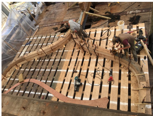
The larger frames are assembled close to their place in the ship's structure. This frame will be at the break in the deck, about mid-ship.
