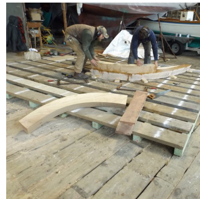
The futtocks are joined into the double-sawn frame and will be fastened with trunnels.
